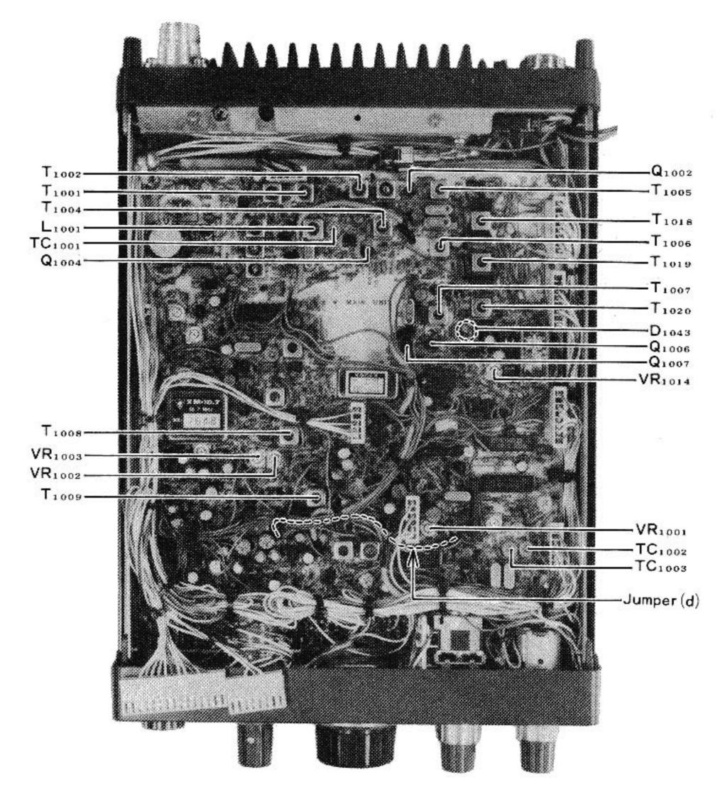
ALIGNMENT AND TEST POINTS FOR RECEIVER
