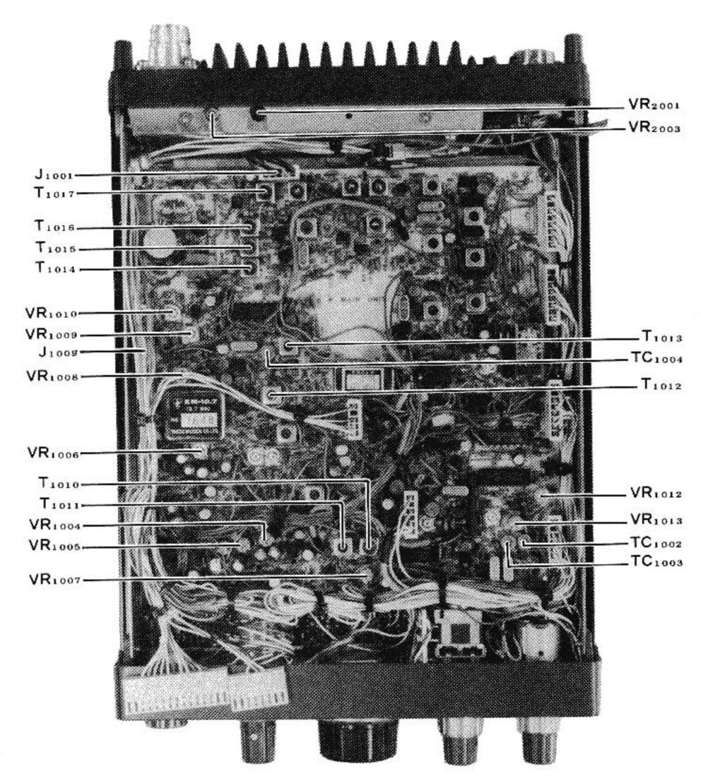
ALIGNMENT AND TEST POINTS FOR TRANSMITTER
