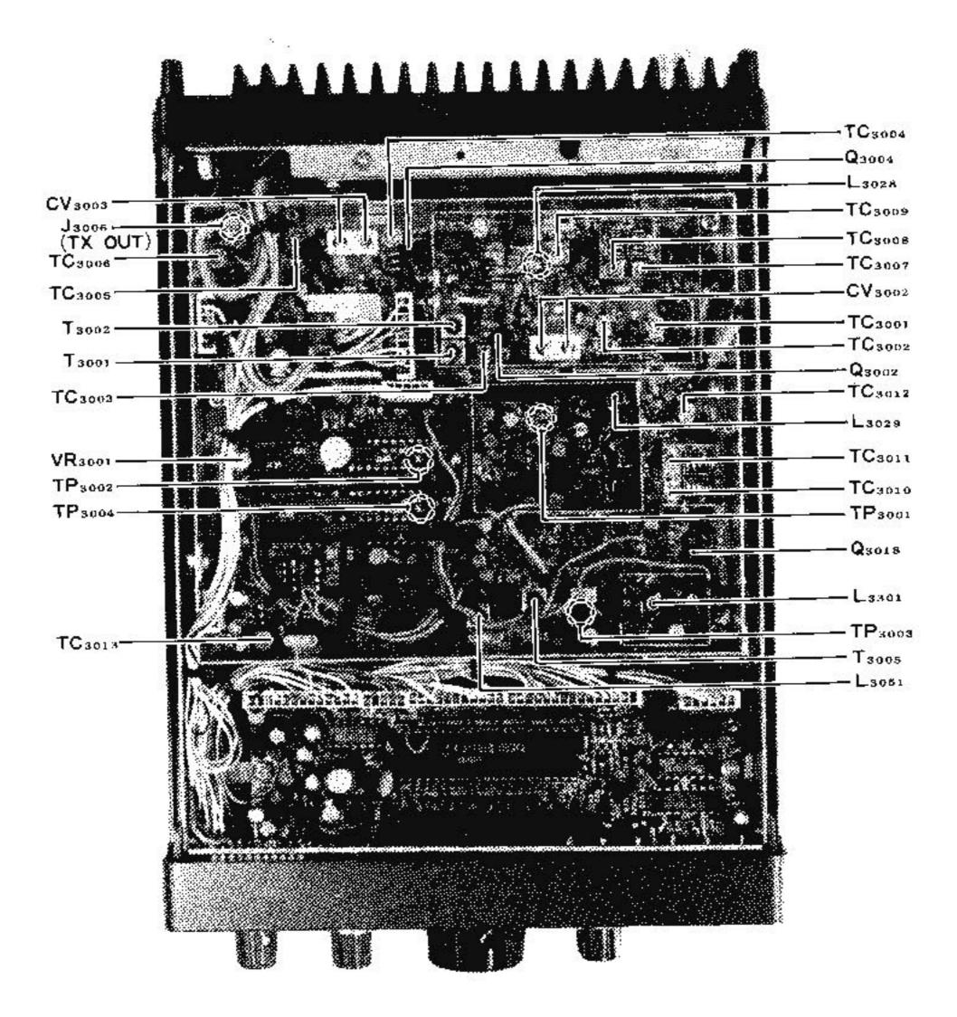
ALIGNMENT AND TEST POINTS FOR PLL
