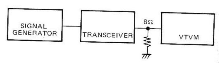
RX SENSITIVITY TEST SETUP
